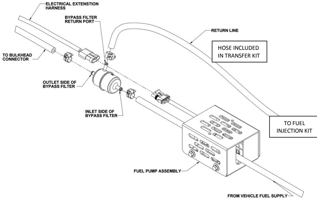
Figure 3. Fuel Pump and Filter Detail
