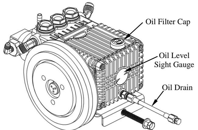
2. After the first **50 hours** of operation, change the crankcase oil with Industrial Pump Oil, (Part # 13-030). Change the crankcase oil every **500 hours** thereafter.
