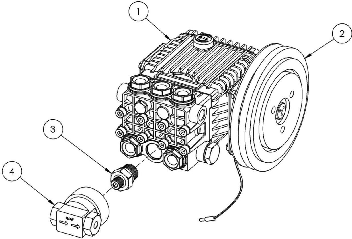
**68-179, ASSY, PRESSURE PUMP (GENERAL PUMP FOR SERIAL #'S 757 AND UP)**
